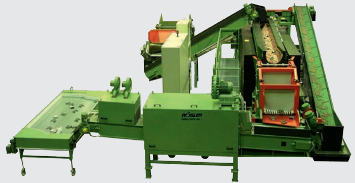
Linear continuous feed finishing system with work piece loading, vibratory feed hopper with weighing cells and loading belt, hot air belt dryer, cooling station, work piece buffer station.
