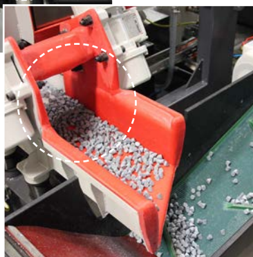
Lower vibratory cross conveyor with residual water screen segment and Media return belt conveyor
