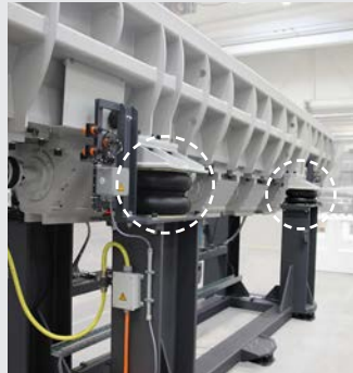
Processing bowl raised at the bowl entrance - shorter processing times
