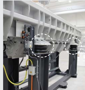
Processing bowl raised at the bowl exit - longer processing times
